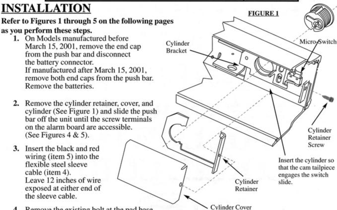
Remove the existing bolt at the pad base end of the link are closest to the key cylinder hole. Slide the 2.75 inch bolt (item 7) provided through the opening of the cable clamp (item 2), and place one end of the flexible steel sleeve cable in the cable clamp (See Figure 5). Replace the 2.75 inch bolt and assembly into the link arm. Replace the washer and nut and secure.
