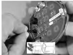
10. Plug the lock cable into the receptacle on the underside of the keypad. Note that the features of the plug and receptacle can only align when the plug is correctly oriented.
