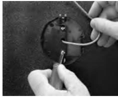
7. Bring the lock cable through the center hole in the mounting base, then fasten the base to the safe door, using either the silver colored pair of 8-32 machine screws or the tinted pair of M4 screws, whichever is appropriate for the prepared holes in the safe door.
