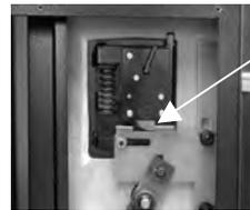
5. The lock cannot function properly if it binds against the safe's boltwork. This photo shows boltwork in the fully locked position, placing pressure on the side of the lock bolt. It could prevent the lock from opening.
