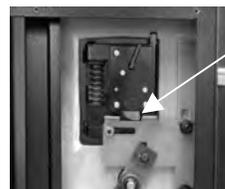
6. In this photo, the boltwork bind has been relieved by removing a small amount of material from the right side of the blocking bar's bolt opening. Now when the boltwork is fully thrown to the locked position, there is air space on all sides of the lock's bolt. This is the desired relationship.
