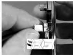
11. If the power leads (red and black wires with white connector) are not already connected to the keypad, plug the white connector into the white receptacle on the back of the keypad. Align the connector's single ridge with the slot in the receptacle.
