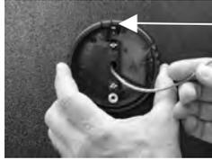
8. Place the keypad ring onto the base. Note that there is a spring-loaded tab at the top of the ring (see white arrow). Orient it as shown when placing the ring on the base.
