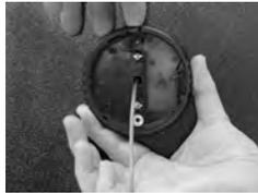
9. Once the ring is against the base, rotate it clockwise until the tab is straight up. You may have to pull the spring-loaded tab forward before you can rotate the ring into position. When the tab is straight up, it will snap into position.
