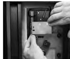
4. If the safe incorporates a relock device plate, it will likely attach to the lock body as shown. If it attaches using the lock's cover screw, make sure the screws engage the lock by at least four threads. Substitute longer 8-32 machine screws if necessary. It may be necessary to trim longer screws to a proper working length. Relock device attaching screws must NOT be longer than the depth of the tapped hole provided in the lock case.
