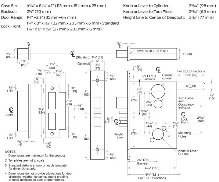
ANSI Standards: L9000-Series locks meet all requirements for installations in doors and frames prepared in accordance with ANSI specifications A156.13, 2012.
